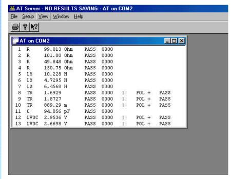
During batch testing, the Server program will present the results of each transformer immediately after it has been tested.
