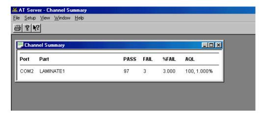
Where a number of AT Series testers are being used, the Database Server also includes the ability to view a 'channel summary'. This display will show live batch summary reports for any of the testers connected to the Server PC
